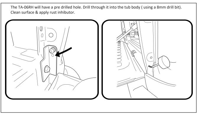
Feed M8 x 20mm button bolt supplied through the bracket and ute body, fasten using the 3mm washer and M8 nyloc nut provided.
