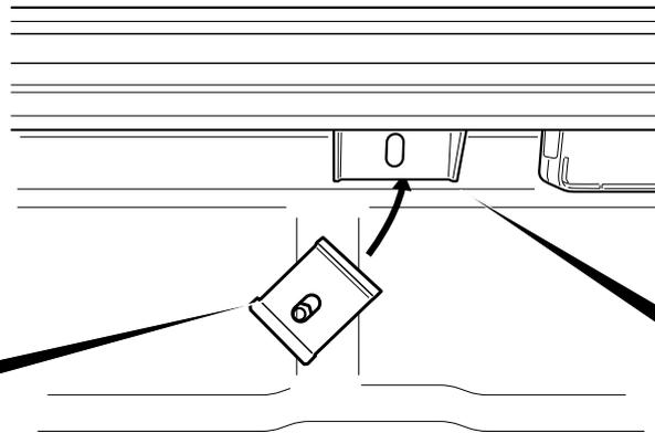
Fasten clamp loosely into position using M8 washer, M8 spring washer and M8 x 35mm bolt.
