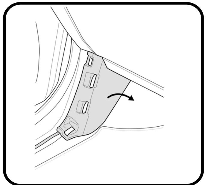
Unplug indicated wiring and plug NP-PATCH wiring.
