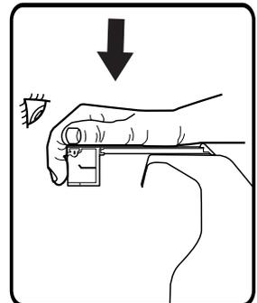
Apply flat plate behind adjusting bolt hole to the ute bed panel or to the liner if the Ute is equipped with a tub liner.
