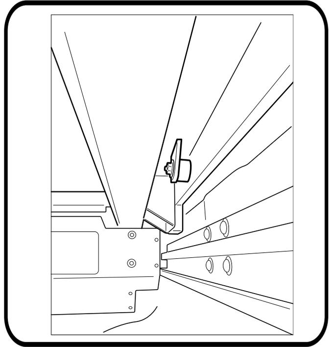
Feed brake light loom back through the cavity and reconnect to connectors for correct operation of brake light.
