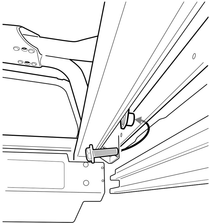
Using the provided M8 hex bolt followed by the m8 washer, feed through the tub lip, nylon space and the sports bar leg. repeat to on the other side.
