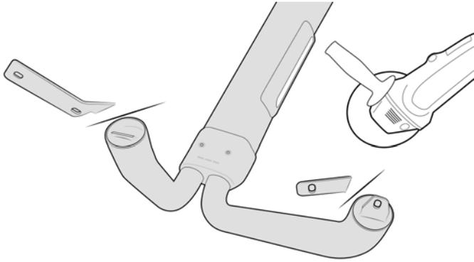
Cut the rear leg as shown be careful not to damage the sports bar.
