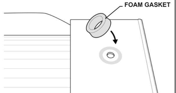
Peel away backing from foam sealant and stick to side rail. Front and rear gaskets are not identical.
