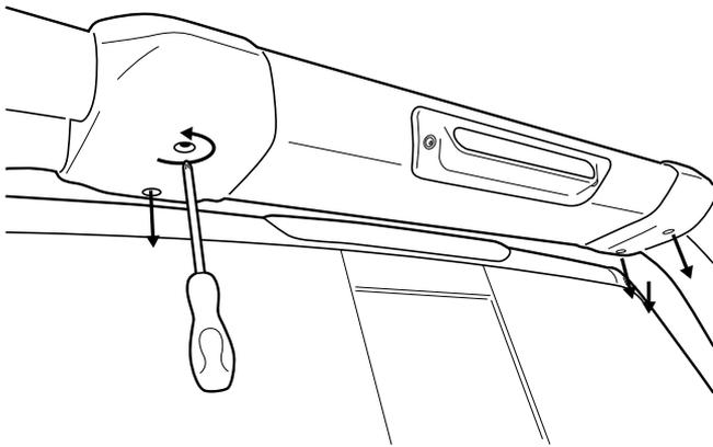
**Remove screws holding plastic cover and retain.**
