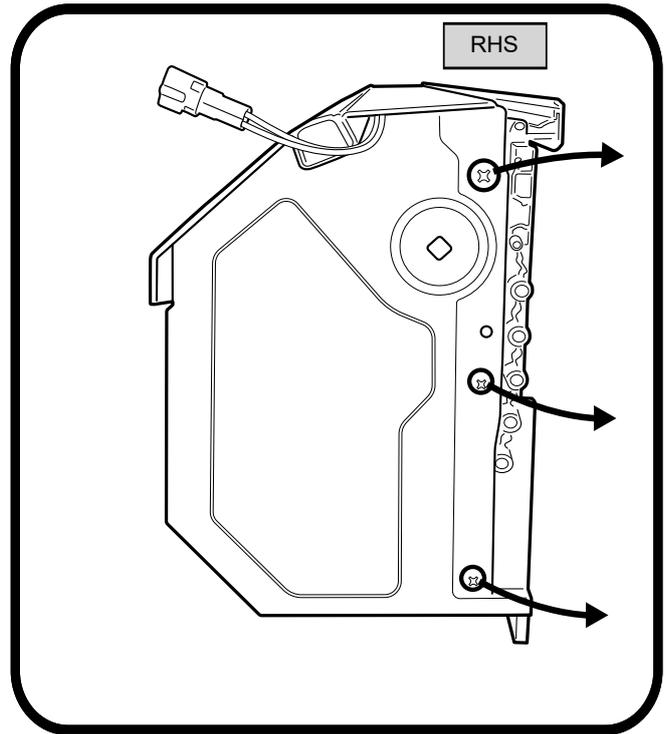
Now on the other side, remove and retain the 4 screws from the canister as indicated.
