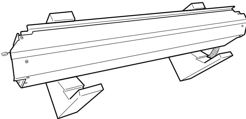
Disengage motor from the axle by unfastening the 3 Screw as indicated. Retain all parts.
