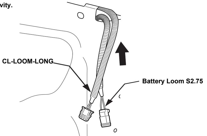
Run cl-loom-long to front passenger door over chassis rail. Cable tie wiring every 500mm.
