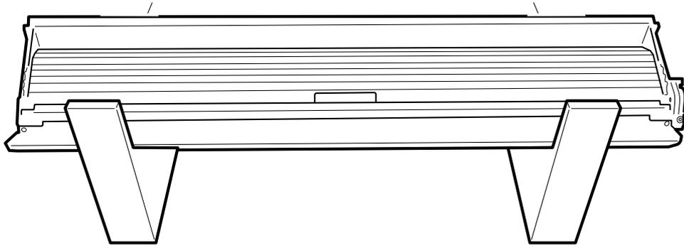
With assistance turn the canister on its back on the foam blocks.
