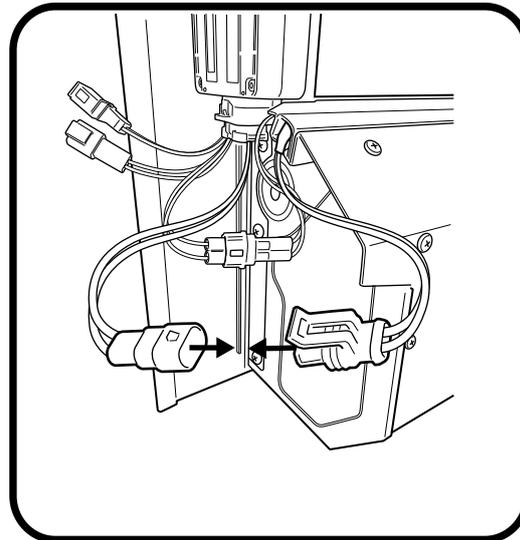
Align side rail to side of canister, guide the track to go in between the curtain end robber stop.
