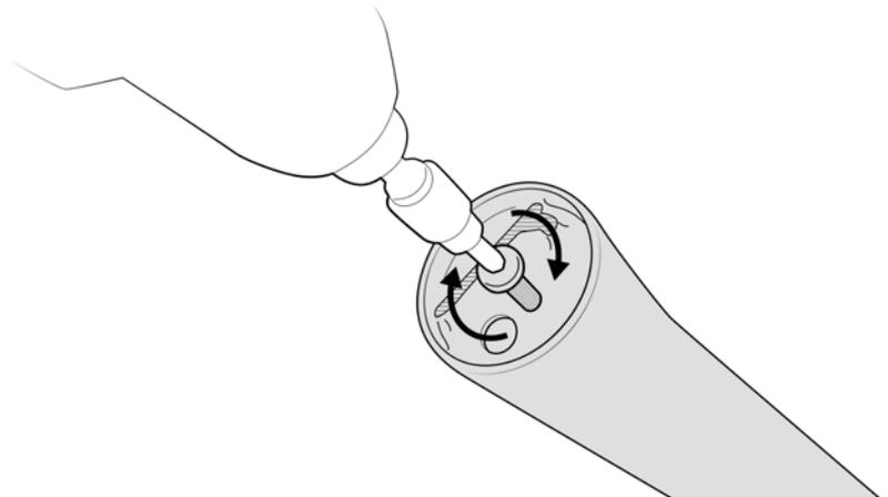
Place and tighten grub screw followed by locking it with the nut.
