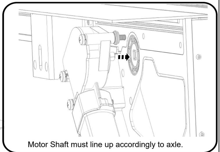
Fasten all 3 screws to 2nm torque. Over tensioning will cause operating issue's.
