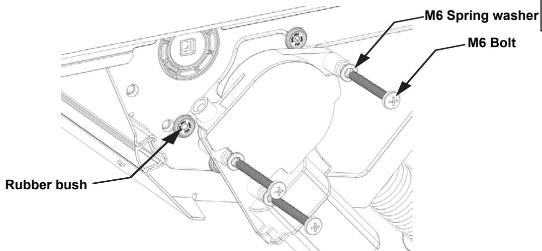
Align & insert motor shaft to axle.
