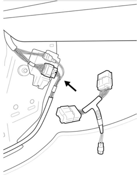
Plug CL-LOOM-LONG to PATCH wiring.
