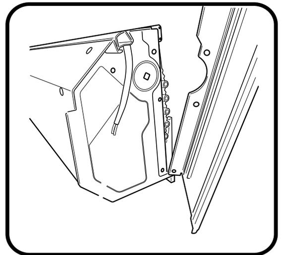
Fasten the side rail using the retained screws, spring washer and washer, only to the locations indicated.
