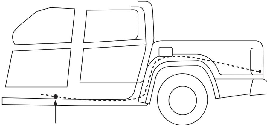
Make a small hole under the front passenger side rail. Be sure to check for obstructions on both sides. Run wiring through small hole made.
