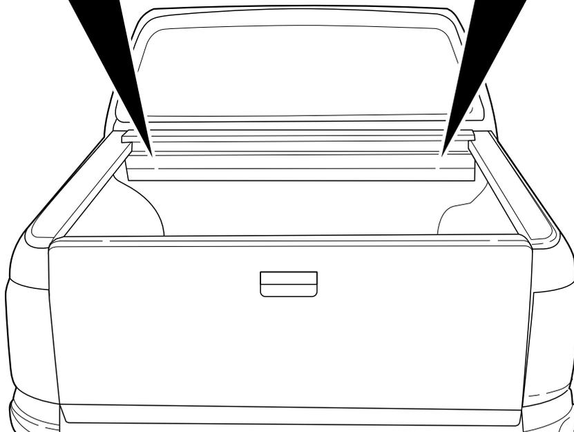
Insert the nylon spacer , repeat step on the other side.
