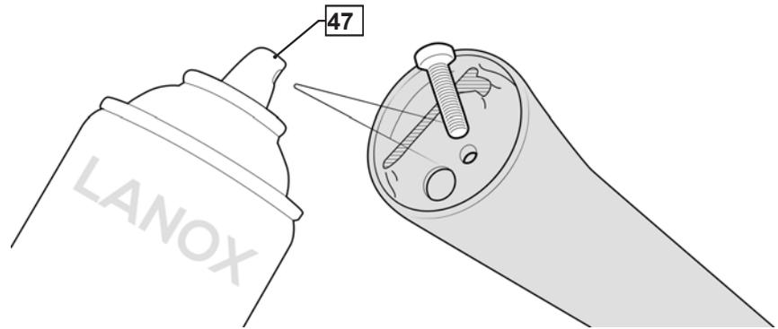
Carefully fasten the threading bolt as shown. This will make a bigger thread in the housing.
