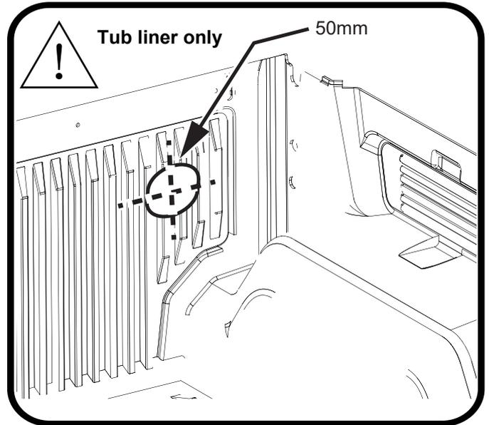
Measure down from top of headboard 225mm & 65mm from inside wall of bed as shown. Repeat to the other side.
