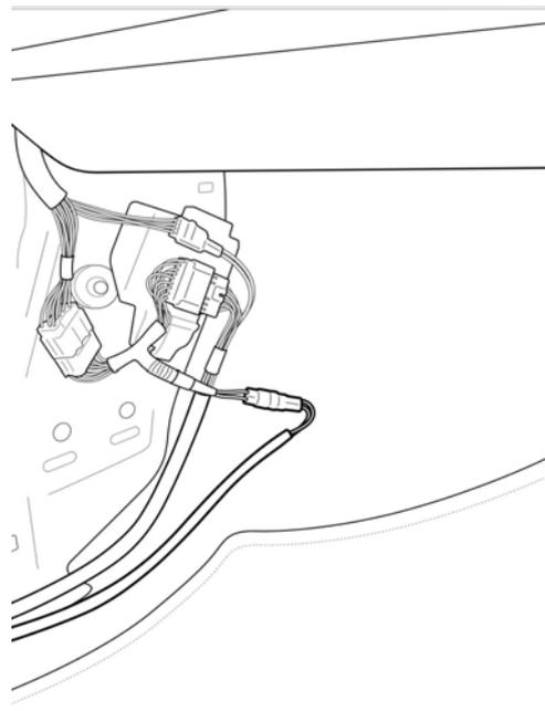
Seal any area where there was an incision or a hole made to have the loom feed in to the cab.
