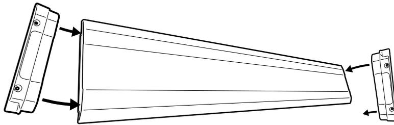
Place & Align top cover over the canister and side rails.
