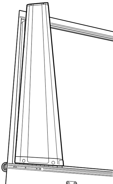
Using countersunk screws provided, line up end cap holes to the threads on the side rail. Fasten to 3nm torque. Repeat to the other side.
