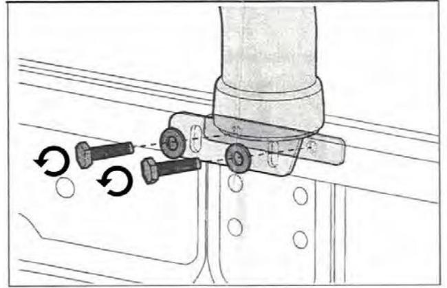
**Remove nuts & bolts holding the sports bars to the vehicle. Discard the removed hardware.**
