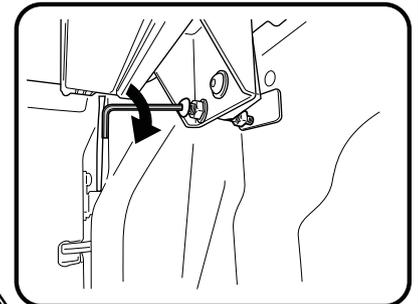
Drive the adjustment bolt in to lift the rear of the side rail till it clears the tailgate.
