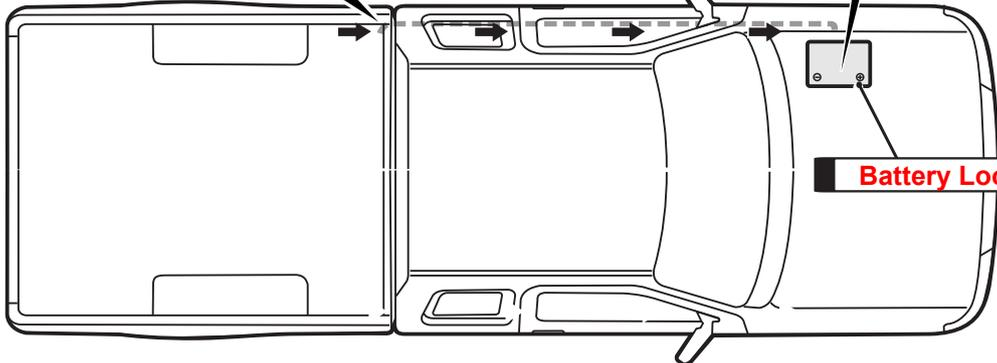
Run the wiring from the front corner cavity ( leaving 200mm in the tub) to the battery over the chassis rail. Making sure to keep away from hot obstructions and cable tie every 400mm. Reconnect fuse patch to battery loom S2.75, now attach fuse patch to positive of battery and earth to the body of the Ute.
