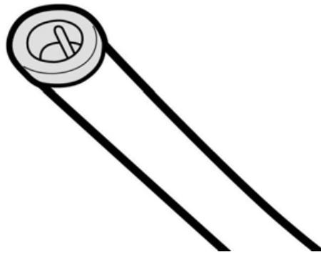
Drill the M6 Sports bar hole with a 6.5mm drill only for the front leg. Repeat for mirroring side
