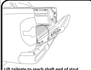
Lift tailgate to reach shaft end of strut, then push in to position.
