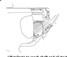
Lift tailgate to reach shaft end of strut, then push in to position.
